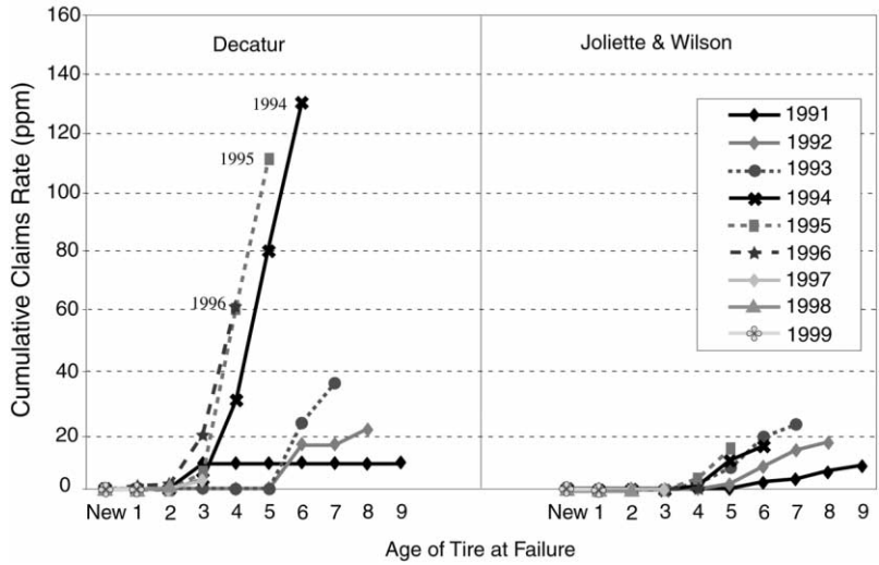
FIG. 2.—Complaints registered by the NHTSA per million P235/75R15 Firestone tires produced, by age of tire, production year, and plant (nonimputed data). Source: Authors' calculations based on NHTSA and Safety Forum data. Complaints concern defects in 1991–99, reported prior to August 2000. Observations with missing data are excluded.
